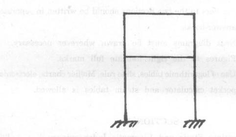
(b) Find slope at 'C' and maximum deflection. Take flexural rigidity =  $4 \times 10^4 \text{ kNm}^2$ . [8]
