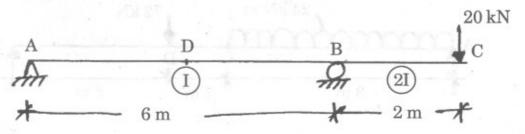
(c) Using Castigliano's first theorem, determine deflection of overhang end 'A' of the beam loaded as shown below. [8]
