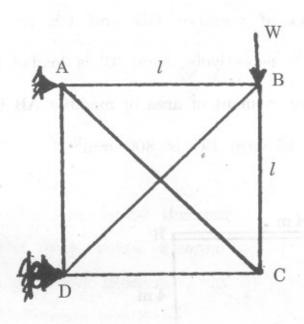
6. (a) Find horizontal deflections of joint 'C' of the pin jointed truss. The area of horizontal members is  $150 \text{ mm}^2$  and the areas of members AC and BC are  $200 \text{ mm}^2$  each. Take  $E = 200 \text{ kN/mm}^2$ . [8]
