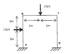
Q5) Analyze the truss by Flexibility Method (EI Constant).
