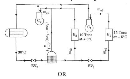
Q6) a) A 25 TR two stage VCRS with flash chamber -as flash gas removal operates with ammonia as refrigerant. The evaporating and condensing temperature are -30°C and 40°C respectively. Estimate COP and power input.
