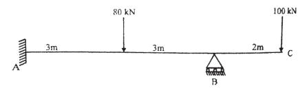
b) Analyse the continuous beam shown in figure below using the Flexibility method and draw the bending moment diagram. [10]
