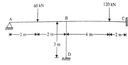
Q5) a) Analyse the frame shown in figure below by portal method.
