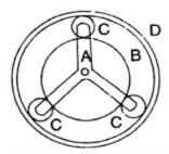
Q4) Fig. shows diagrammatically a compound epicyclic gear train. Wheels A,D and E are free to rotate independently on spindle O, while B and C are compound and rotate together on spindle P,on the end of arm OP. All the teeth on different wheels have the same module. A has 12 teeth has 30 teeth and Chas 14 teeth cut externally. Find the number of teeth on wheels D and E which are cut internally.
