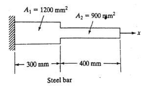
Assume Modulus of Elasticity E = 210 GPa and Density ( $\rho$ ) = 7800 kg/m<sup>3</sup> OR
