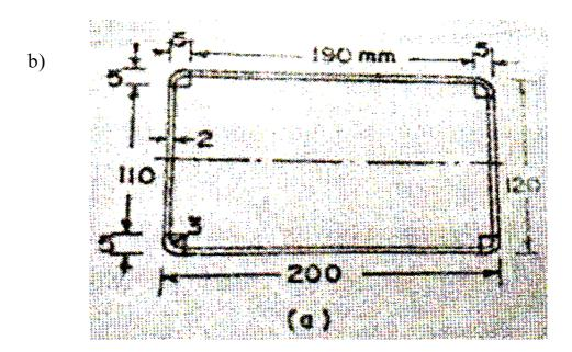
Find the allowable load for the rectangular tubular column section show in fig. The effective length of column is 3.3 m.Take fy=235N/mm<sup>2</sup>. [15]
