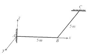
b) Derive the transformation matrix for the two noded grid element. [6]
