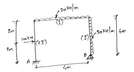
Q5) a) Determine the approximate values of moment, shear & axial forces in member of the frame loaded & supported as shown in figure using cantilever method of analysis.[12]
