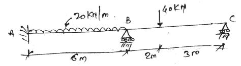
b) Analyse the continuous beam shown in figure using flexibility method & draw the bending moment diagramme. [10]
