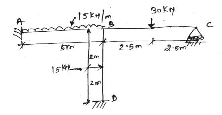
b) Analyse the continous beam shown in figure by moment distribution method. Draw BMD & SFD. [10]
