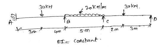
Q3) Analyse the beam shown by stiffness matrix method. Draw BMD & elastic curve. EI = constant. [16]
