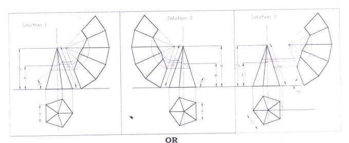
Q.8) A cone of base 40 mm diameter and height 60 mm rests on its base on H.P. A sectional plane perpendicular to V.P and inclined at 35° to H.P passes through the point on axis at 35 mm above HP. Draw the development of the lateral surface of the truncated cone. [12 marks]
