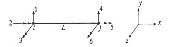
b) Derive the transformation matrix for the two noded grid element. [6]
