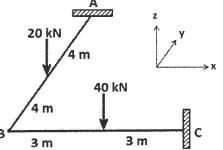
**Q7)** The tripod shown in figure is subjected to horizontal and vertical loads. Determine the deflections at the loaded joint using stiffness matrix method. Take E = 200 GPa and c/s area of all members 1000 mm<sup>2</sup>. [16]
