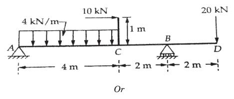
2. (A) The beam is supported and loaded as shown in figure. Draw SFD and BMD indicating all important values. [6]
