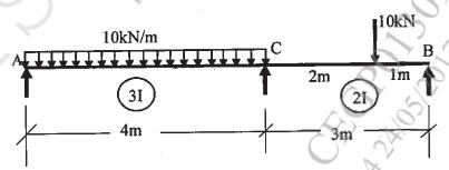
Q2) a) Find slope and deflection at point 'B' for cantilever beam by conjugate beam method [6]
