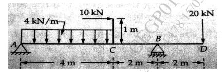
Q.2 A) The beam is supported and loaded as shown in figure. Draw SFD and BMD indicating all [06] important values.
