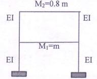
Q. 5) Derive the formulae for modal masses and modal stiffness for two Degree of Freedom System [13 marks]
