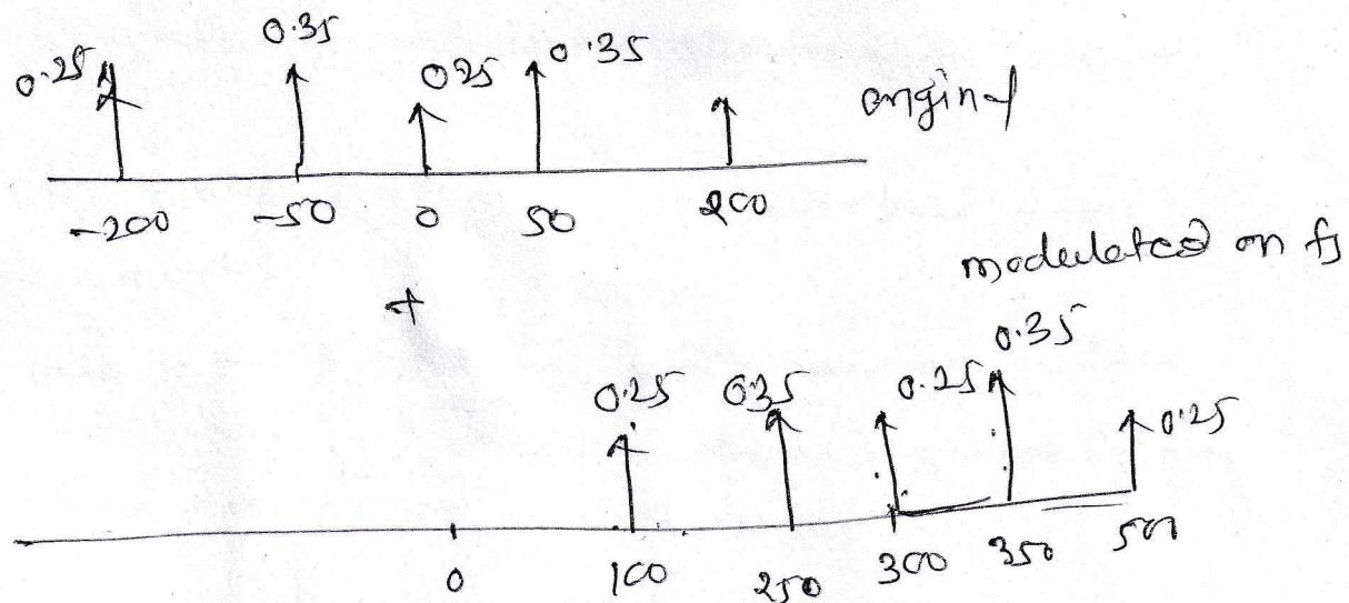
complete spectrum is addition of original + modulated on  $f_s$
