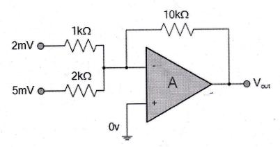
d) If  $V_1$ = 2V and  $V_2$  = 1.5V, calculate the output voltage. Also calculate output for the values of  $V_1$ = -2V and  $V_2$  = 4V.
