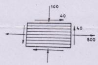
$E_1 = 150 \text{ kN/mm}^2, \ E_2 = 12 \text{ kN/mm}^2, \ G_{12} = 7 \text{ kN/mm}^2, \ v_{12} = 0.2, \ X_t = 1550 \text{ N/mm}^2, \ X_c = 1150 \text{ N/mm}^2, \ Y_t = 60 \text{ N/mm}^2, \ Y_c = 240 \text{ N/mm}^2, \ S = 75 \text{ N/mm}^2$
