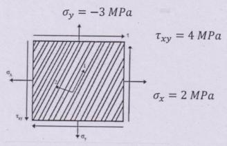
b) A carbon epoxy unidirectional lamina is subjected to a stress system as shown in Figure (stress are N/mm²). The ply properties are [6 marks]
