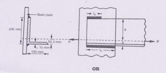
Q.6 a Derive the procedure in the design of bolts for eccentrically loaded bolted joints [4 Marks] in shear.
