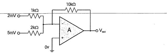
d) For a given circuit diagram, if  $V_1 = 4V$  and  $V_2 = 1.5V$ , calculate the output voltage Vout. Also calculate output voltage Vout for the values if  $V_1 = -1V$  and  $V_2 = 3V$ .
