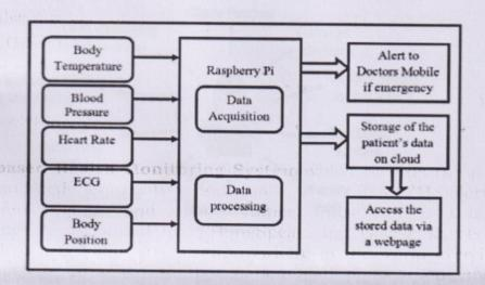
Block diagram is shown in figure. The diagram is into parts: Transmitter and receiver. transmitter In the section all the sensors are connected to the raspberry processor which does acquisition and processing and the processed data in the database which is on cloud. In the receiver section a web page is built and data collected displayed on the web page by an authorized person. Also, the doctor is alerted in case of emergency.
